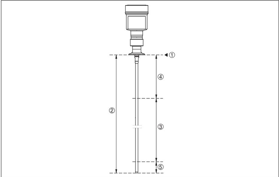
Fig. 34: Measuring ranges - SITRANS LG240
