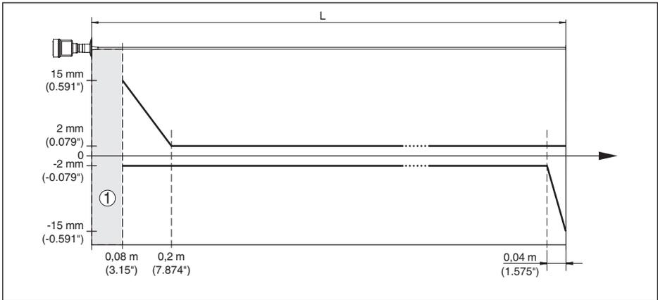
Fig. 35: Deviation SITRANS LG240 in rod version in water
