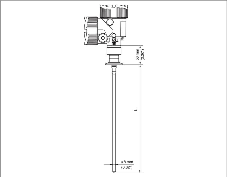
*Fig. 39: SITRANS LG240, rod version  $\varnothing$  8 mm (0.315 in), polished*
