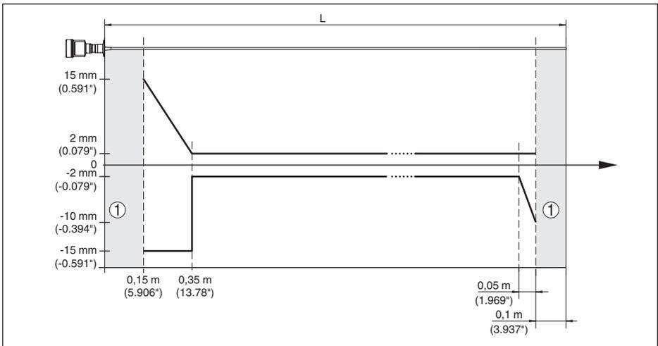
Fig. 36: Deviation SITRANS LG240 in rod version in oil
