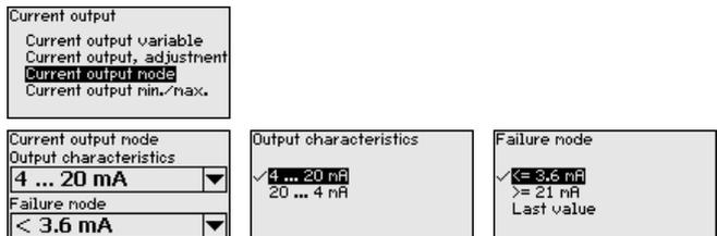
The default setting is output characteristics 4 ... 20 mA, failure mode < 3.6 mA.
