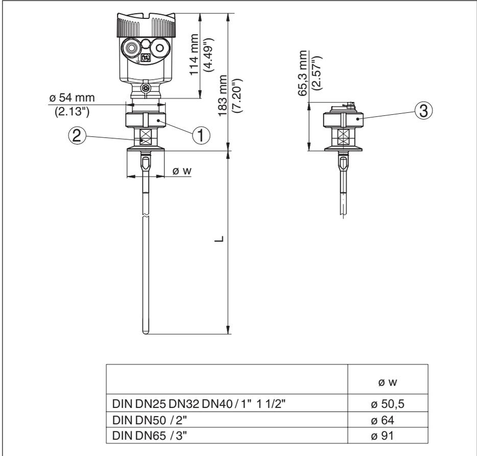
Fig. 40: SITRANS LG240, rod version  $\varnothing$  8 mm (0.315 in), polished - autoclaved version
