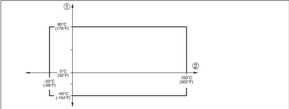
Fig. 37: Ambient temperature - process temperature, standard version
