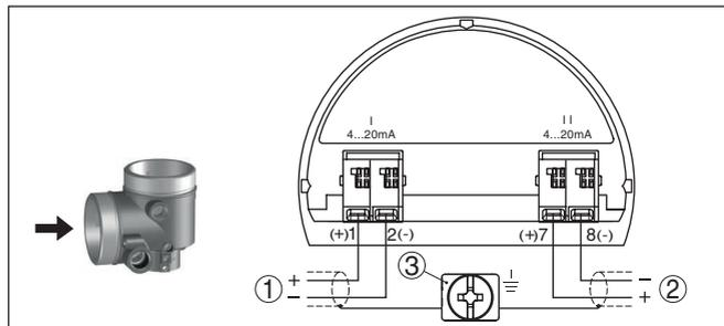
Fig. 15: Connection compartment double chamber housing, supplementary electronics - second current output
