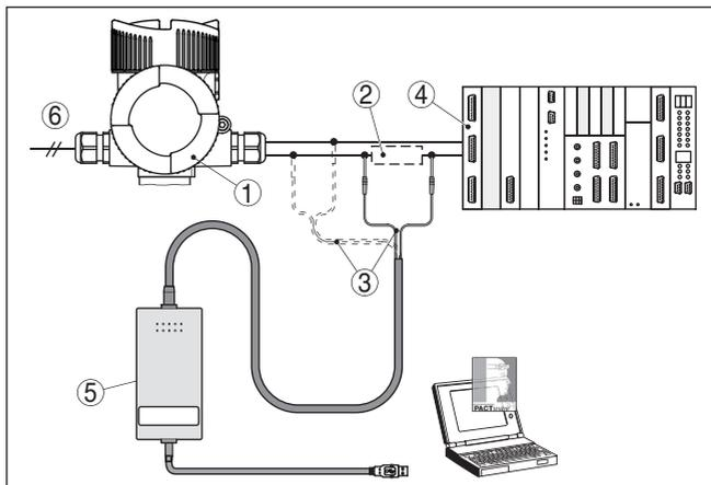
Fig. 20: Connecting the PC via HART to the signal cable
