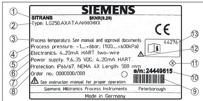
Fig. 2: Layout of the type label (example)
