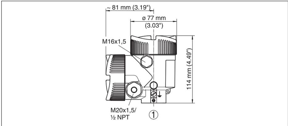
Fig. 38: Dimensions housing - with integrated display and adjustment module the housing is 9 mm/0.35 in higher
