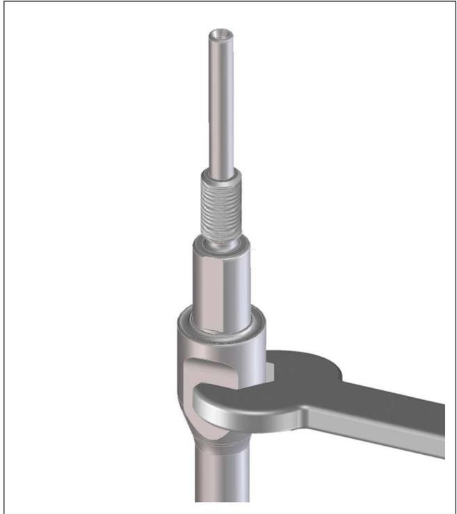
Fig. 33: Exchanging the measuring rod
