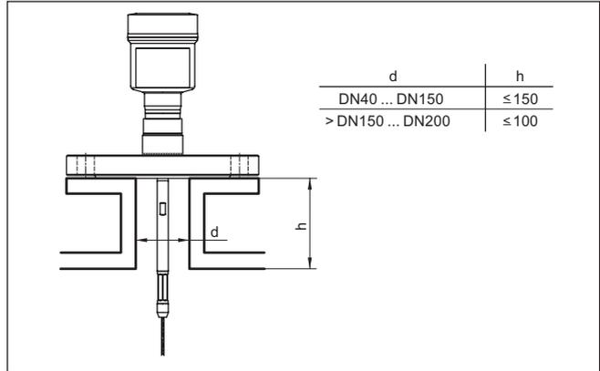
Fig. 7: Mounting socket
