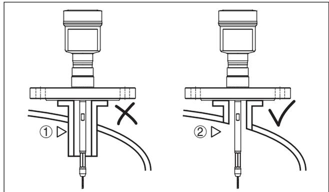
Fig. 8: Socket must be installed flush
