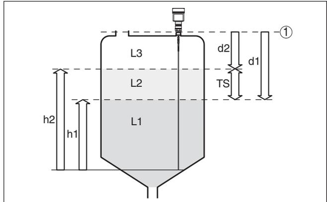
Fig. 4: Interface measurement
