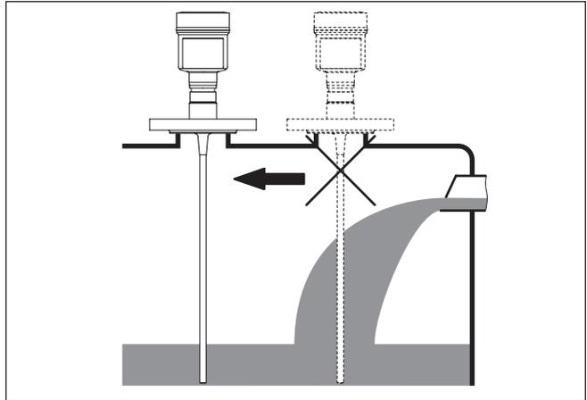
Fig. 9: Mounting of the sensor with inflowing medium
