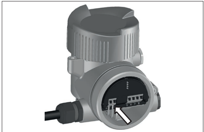
Fig. 11: Connection steps 5 and 6 - Double chamber housing
