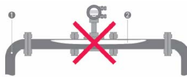
Bad installation, vapor may be trapped in high point of piping
