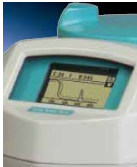
Echo profile shown on integral LCD display
