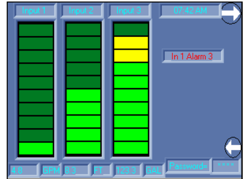
Main screen displays bar graph and digital value, as well as alarms
