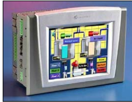
Advanced Controller with integral 5.7" color touch screen
