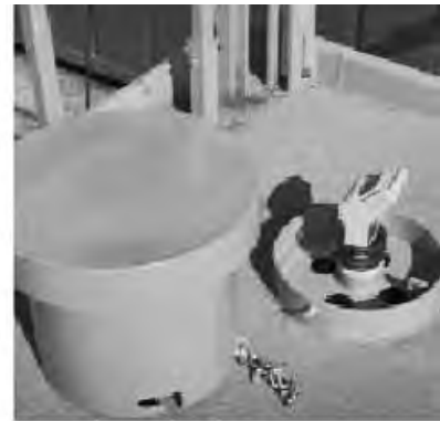
Drilling mud pits
