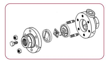
The simple design of the sliding gate valve eliminates most maintenance problems, and those that may be required are easy to perform. Disassembly of the valve is very simple and, since the seats are not welded to the stem, they conveniently lift out of the body. Should your flow requirements change, interchangeable Cv's are available in flow coefficients as low as 0.0008 and as high as 395 (depending on body size).
