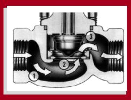
In conventional rising stem globe style valves, the flow changes directions three times as it follows an "S" path. This leads to greater velocity, turbulence, noise and more wear on the seating components.
