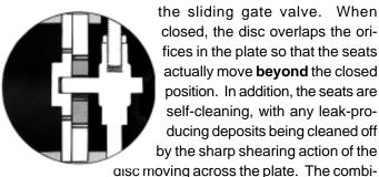
the sliding gate valve. When closed, the disc overlaps the orifices in the plate so that the seats actually move beyond the closed position. In addition, the seats are self-cleaning, with any leak-producing deposits being cleaned off by the sharp shearing action of the
